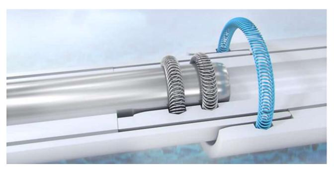
BAUMANN Contact Elements are springs that protect systems and components from electromagnetic interference (EMI). The spring acts as sealing that transmits current between the male and the female part of a connector. Various interface designs, materials and coatings are available. In addition to favorable electrical and mechanical properties described under Electricial contact and Mechanical retention, BAUMANN Contact Elements have advantageous shielding properties:
